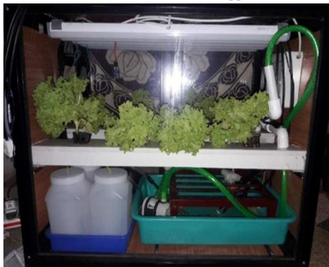
Figure 4 : HydroponicsSystem Prototype with Lettuce
