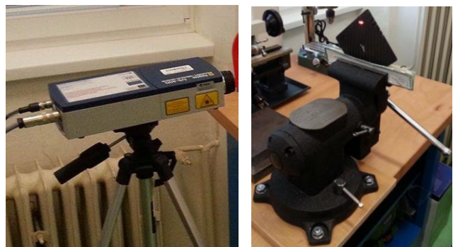
Figure 3. Laser vibrometer Polytec (a), jaw clamping of sample (b)
