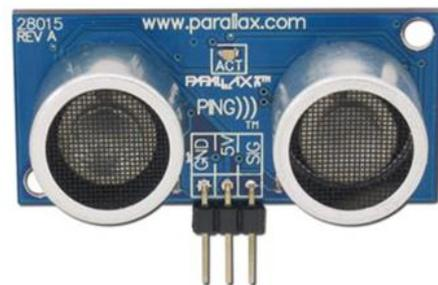
**Figure 10.**Ultrasonic Sensor
