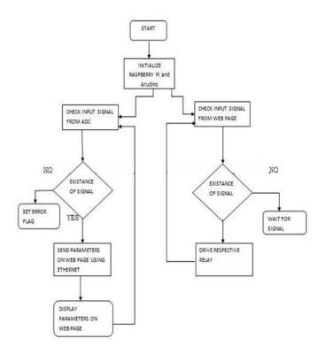
ALGORITHM USED FOR SMART FARM MONITORING USING RASPBERRY PI AND ARDUINO
