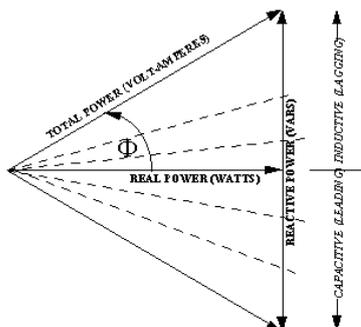
In certain cases there would be deficient reactive power,hence reactive power should be added to meet the required reactive power factor. In such a case FACTS is the solution where it as a inductive circuit. Effect of reactive power
