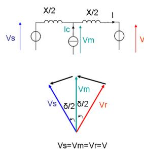
In shunt compensation, the controller (variable impedance or variable voltage source or combination of both) is parallel to the system. FACTS works as a
