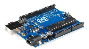
forward. The Uno is the latest in a series of USB Arduino boards, and the reference model for the Arduino platform.
