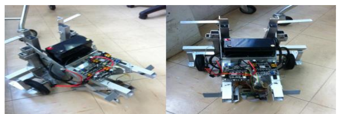
Figure 6. Side angle view and top view of robot mechanism with hardware and components attached
