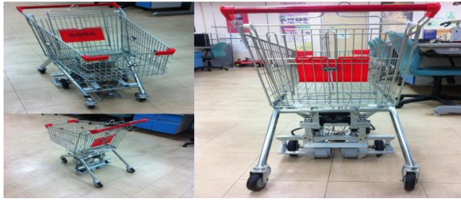
Figure 7. Mechanical structure of portable robot is attached to shopping trolley.
