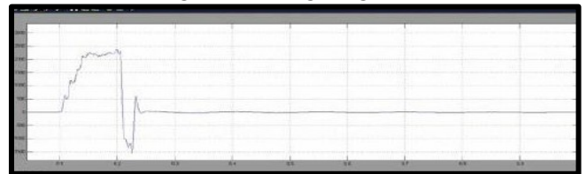
Figure 5. The simulation waveform of the load voltage for voltage sag of 27%
