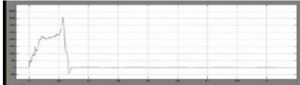
Figure 8. Simulation waveform for per phase error voltage 3 in RMS value
