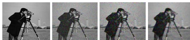
Figure 6. (a) Original image 5 (Cameraman), (b) Image with 30% impulse noise, generated using two-sided fixed impulse noise model, (c) Filtered output of ANCLPVMF, (d) Filtered output of PROPOSED METHOD.
