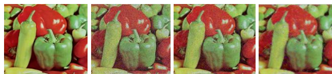
Figure 5. (a) Original image 4 (Pepper), (b) Image with 30% impulse noise, generated using two-sided fixed impulse noise model, (c) Filtered output of ANCLPVMF, (d) Filtered output of PROPOSED METHOD.
