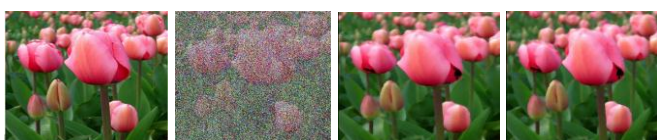
Figure 4. (a) Original image 3 (Tulip), (b) Image with 30% impulse noise, generated using two-sided fixed impulse noise model, (c) Filtered output of ANCLPVMF, (d) Filtered output of PROPOSED METHOD.
