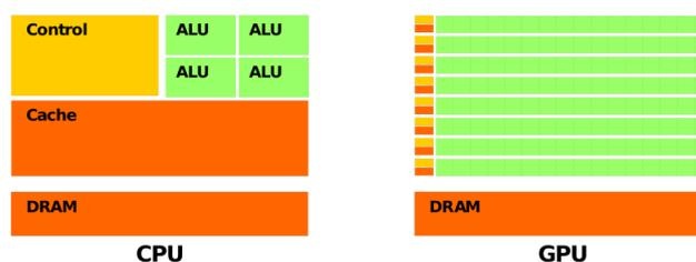
Figure 1. CPU v/s GPU Architecture.
