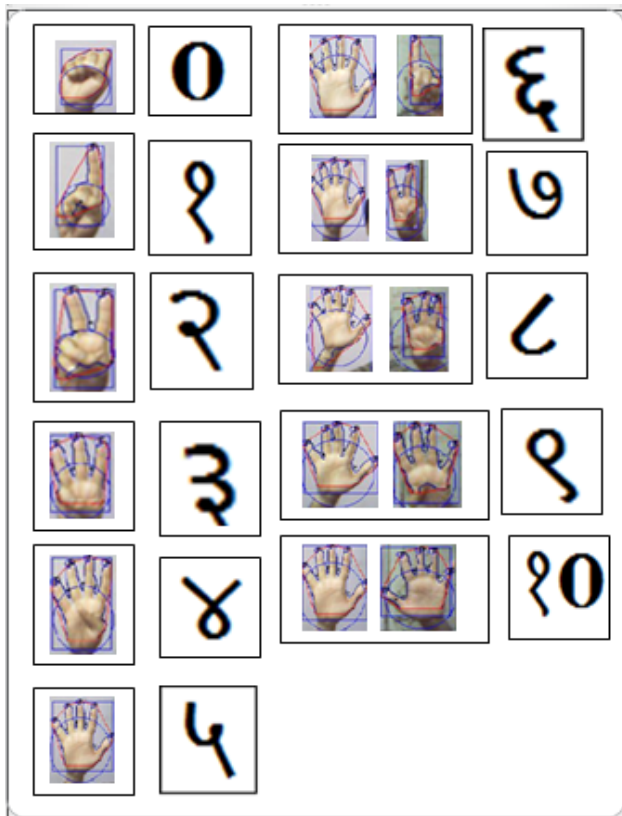
Figure 13. Outcome of RTNDSLTS System as Recognition of DSL Numbers and Corresponding Devnagari Numbers using Fingertip based Recognition Method
