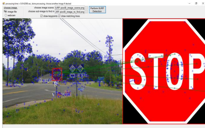
(a) Input image (b) Output of SURF algorithm Figure 3 Feature Extraction by SURF algorithm From Image
