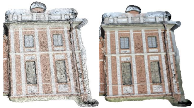
(d) Mesh Surface (left); Textured Surface (right) for \gamma = 2.8 Figure 7. Portion of Reconstructed Surface
