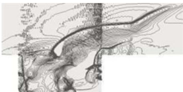
**Figure 7.** Density contour at time,  $t = 0.4$  sec.
