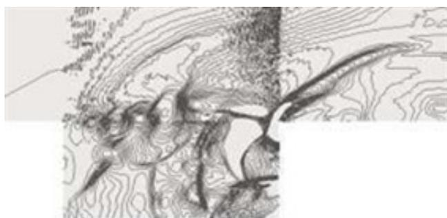
**Figure 6.** Density contour at time,  $t = 0.3$  sec.
