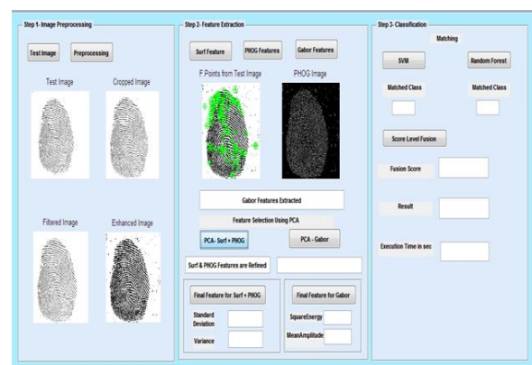
Figure 7. Feature selection process using PCA method by combining SURF and PHOG features.
