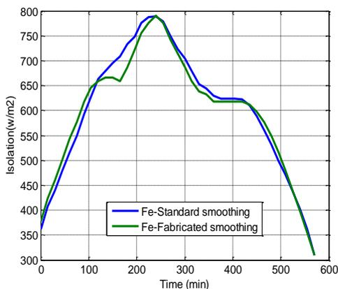
Figure 4. A comparison of the standard and designed pyranometers using Fe
