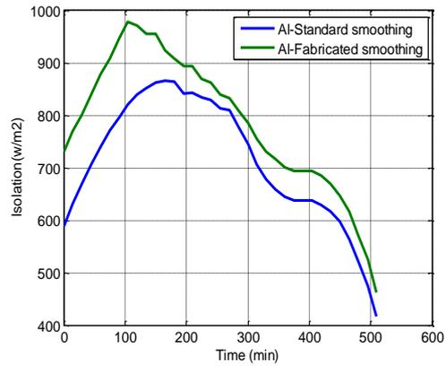
Figure 5. A comparison of the standard and designed pyranometers using Al
