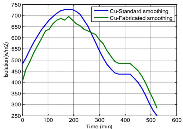
Figure 6. Comparison between the standard and designed pyranometers - Cu
