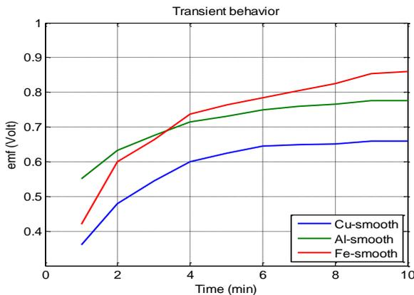
Figure 3. Transient behaviors of three metals
