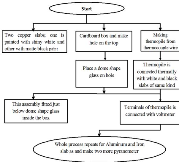
**Figure 1.** Construction method of the novel pyranometer
