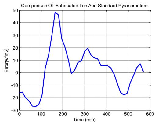
Figure 7. Error between the standard pyranometer and the newly designed pyranometer fabricated by iron slab
