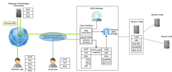
**Figure 3.** The system architecture of “Padova Smart City.”
