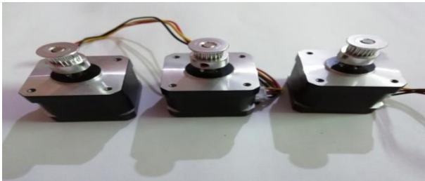
Figure 1. NEMA 17 Stepper Motor
