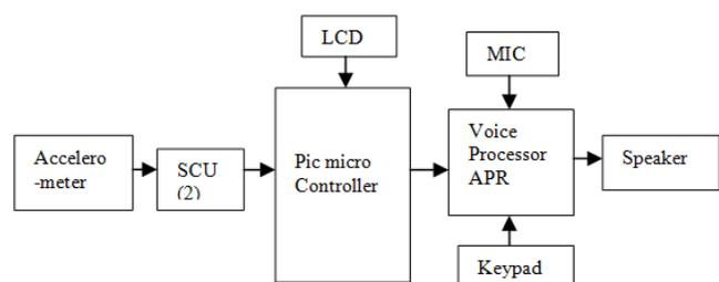
**Figure 2.** block diagram of the hardware proposed method
