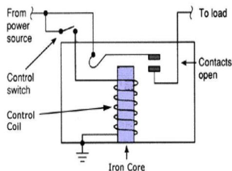
Figure 7. Relay construction
