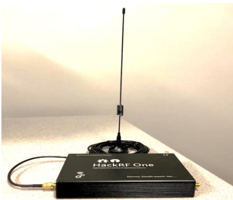
Figure 4.1. Hack RF One| a low cost, open source software defined radio
