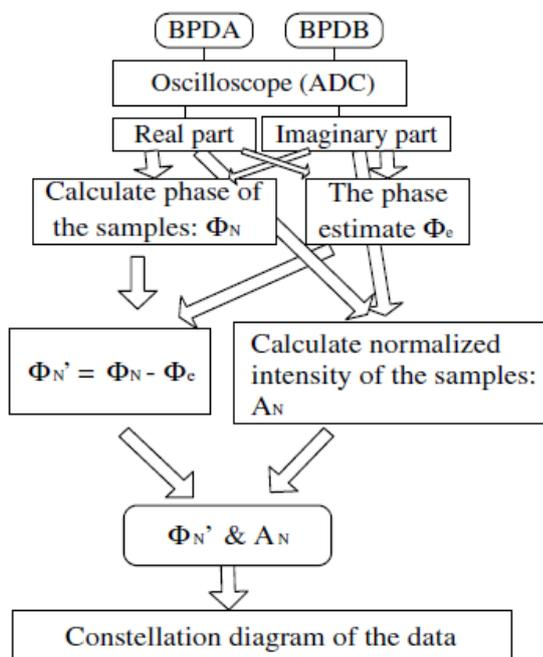
Fig. 2. A block diagram of the signal-processing algorithm.
