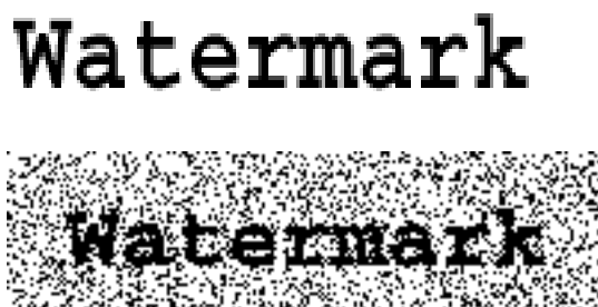
Figure 1. Ideal Watermark-Object vs. Object with 25%Additive Gaussian Noise
