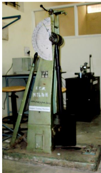
Fig.4 Charpy Impact tester
