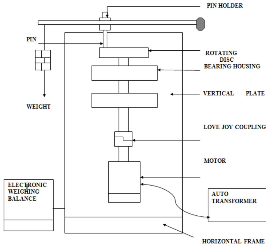
**Figure 1.** Pin on disc wear test apparatus
