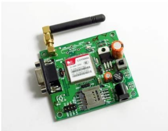
Figure 6. Global system for mobile communication (GSM)
