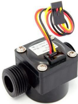
Figure 2. G 1/2 Water Flow sensor
