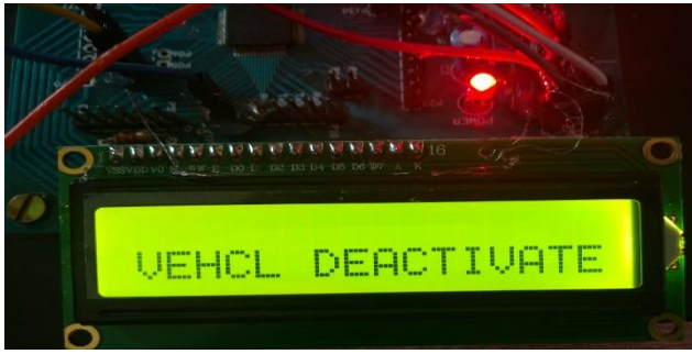
Figure 7. When rider has not worn helmet or alcohol content is detected, the vehicle unit is deactivated.
