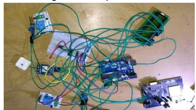
Figure 3. Interfacing of GSM and GPS with Arduino
