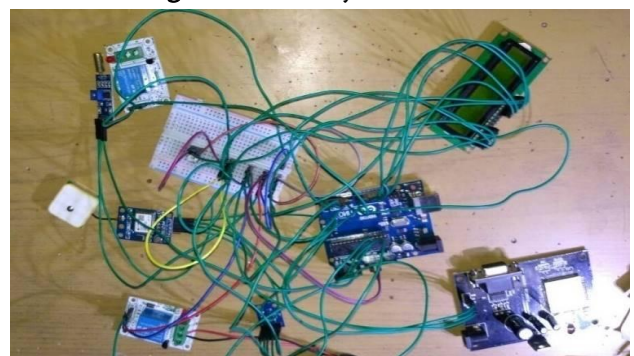
Figure 3. Interfacing of GSM and GPS with Arduino
