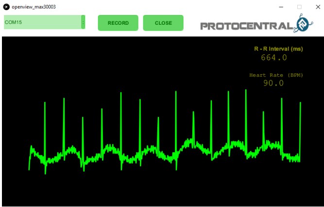
Figure 7. ECG signal acquired through Ag/AgCl electrodes
