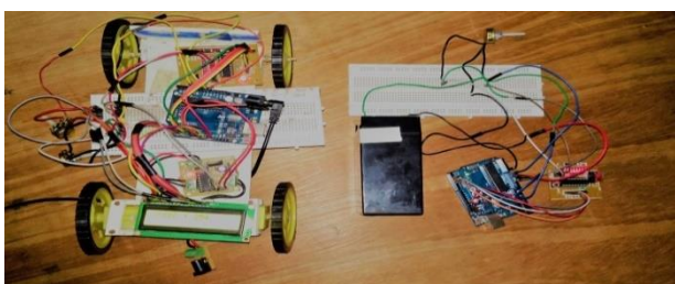
Figure 5. A snapshot of the RF communication system
