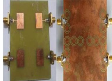
Figure-2 Fabricated Type-I MIMO Antenna
