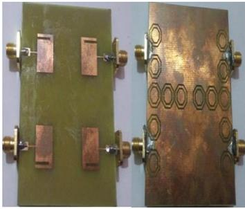
**Figure-5** Fabricated Type-II MIMO Antenna
