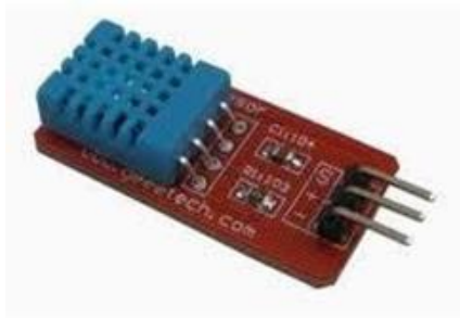
Fig. 3 Temperature and Humidity Sensor DHT11.
