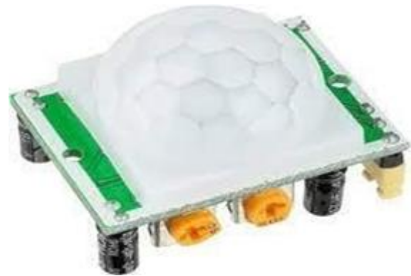
Fig. 5 PIR Motion Sensor
