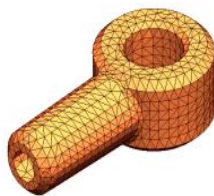
Model subdivided into small pieces (elements)
