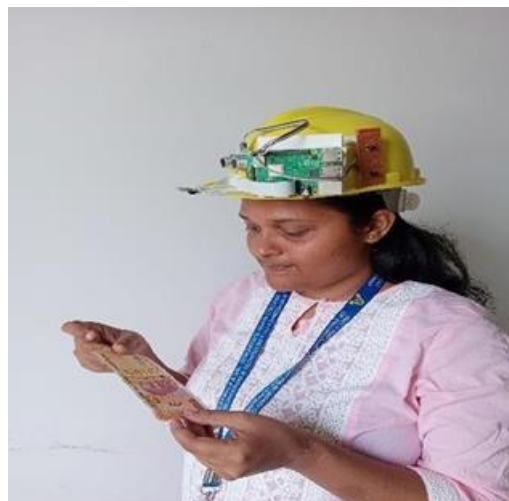
Figure 4. This figure shows women wearing “Smart Cap” that detects the Currency.
