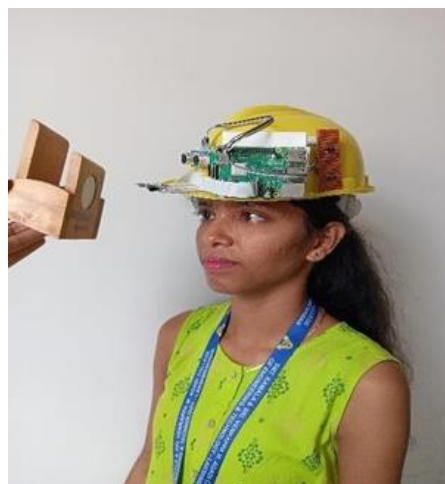
Figure 3. This figure includes women wearing a prototype “Smarts Cap” that detects Obstacle.
