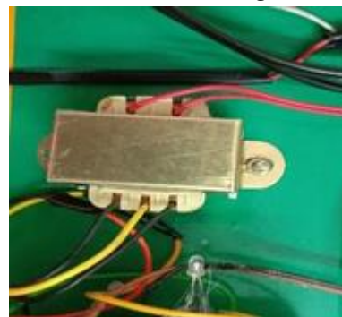
Figure 2: Step Down Transformer
