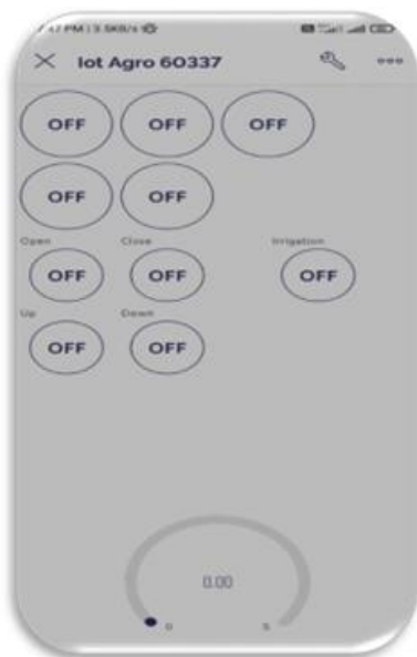
Figure 14: Outfit of All the Functions performed by the Robot using Blynk IOT
