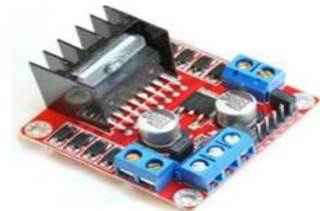
Figure 7: L298N Motor Driver
