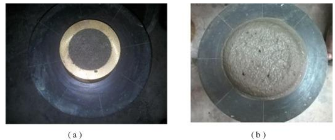
Figure 1. (a) Mortar sample in brass mold, and (b) mortar sample turned to pancake shape
