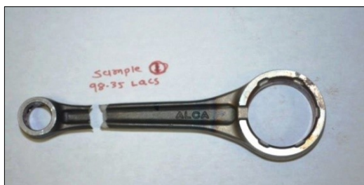
Figure 7.2 Sample ‘1’ Prototype Failed at near to Small End
