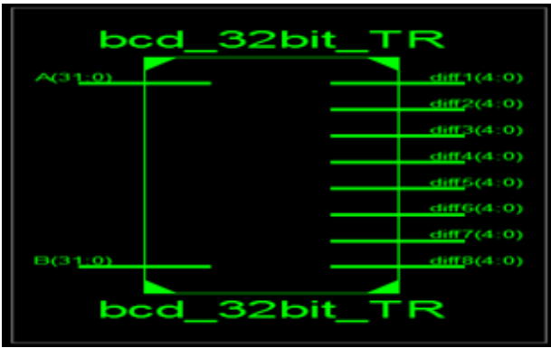
Figure 3.5.1: View Technology Schematic of 32-bit Reversible Adder/Subtractor using DKG Gate
