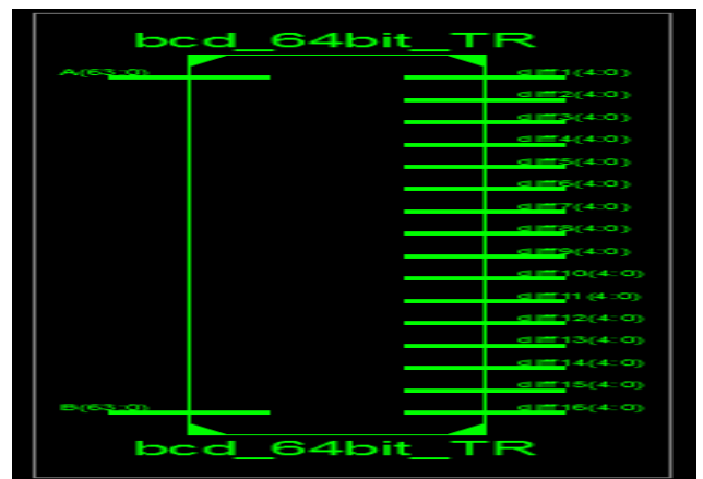
Figure 3.4.1: View Technology Schematic of 64-bit Reversible Subtractor using TR Gate
