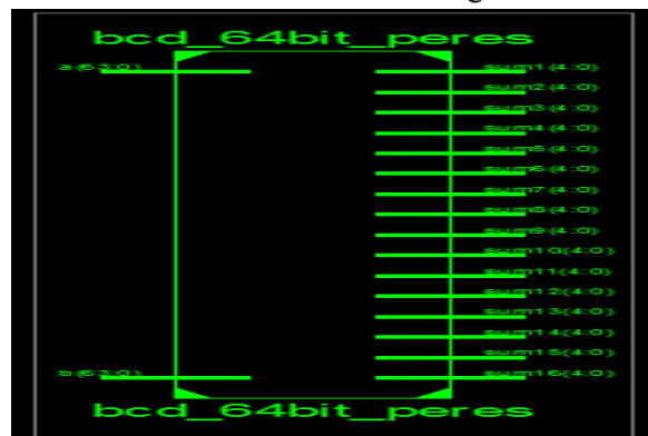
Figure 3.3.1: View Technology Schematic of 64-bit Reversible Adder using Peres Gate
