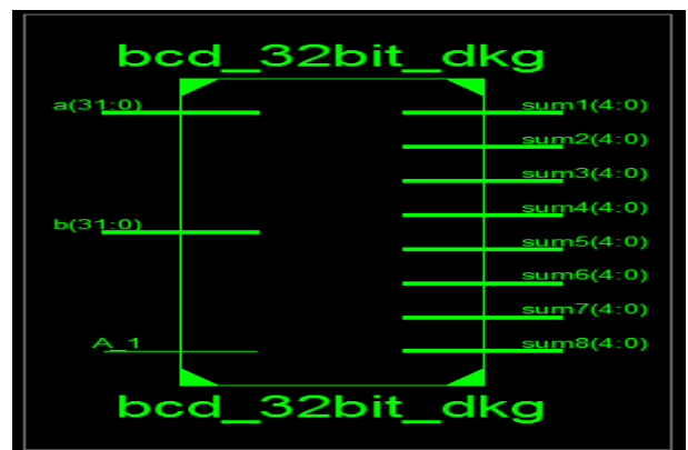
Figure 3.5.1: View Technology Schematic of 32-bit Reversible Adder/Subtractor using DKG Gate
