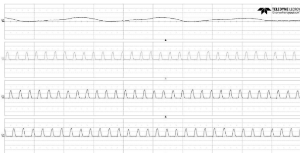
(d) Turn-on angle at 3° and turn-off at 12°
