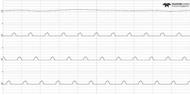
(f) Turn-on angle at 5° and turn-off at 13°
