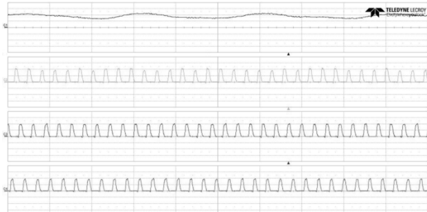
(b) Turn-on angle at 1° and turn-off at 11°
