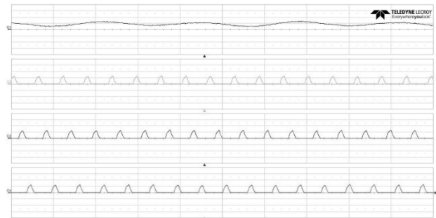
(f) Turn-on angle at 5° and turn-off at 13°
