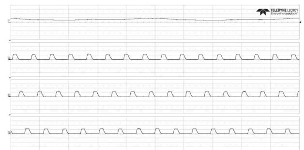
(b) Turn-on angle at 1^\circ and turn-off at 11^\circ
