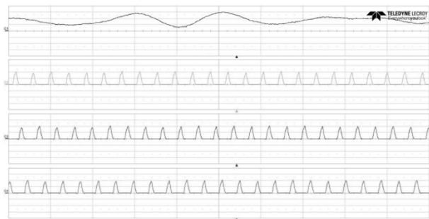
(f) Turn-on angle at 5° and turn-off at 13°
