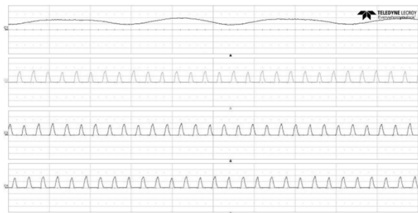
(e) Turn-on angle at 4° and turn-off at 13°
