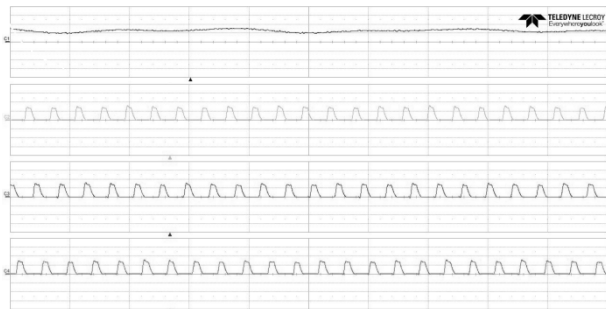
(a) Turn-on angle at 0° and turn-off at 11°
