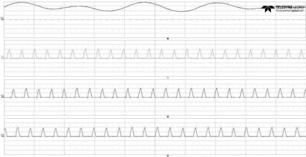
(f) Turn-on angle at 5° and turn-off at 13°
