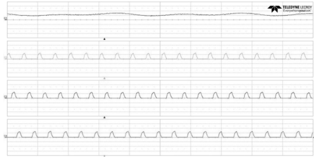
(e) Turn-on angle at 4° and turn-off at 13°
