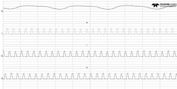
(c) Turn-on angle at 2° and turn-off at 12°
