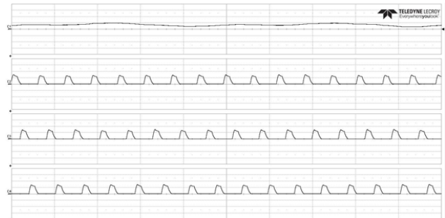
(a) Turn-on angle at 0^\circ and turn-off at 11^\circ
