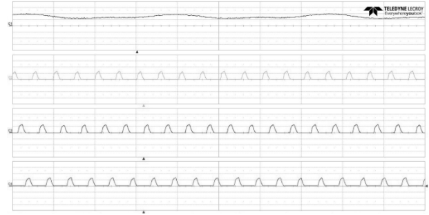
(d) Turn-on angle at 3° and turn-off at 12°
