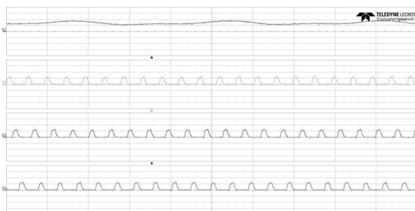
(c) Turn-on angle at 2° and turn-off at 12°
