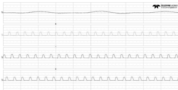
(b) Turn-on angle at 1° and turn-off at 11°
