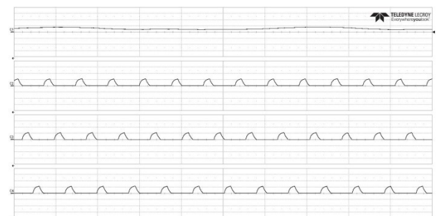
(e) Turn-on angle at 4^\circ and turn-off at 13^\circ
