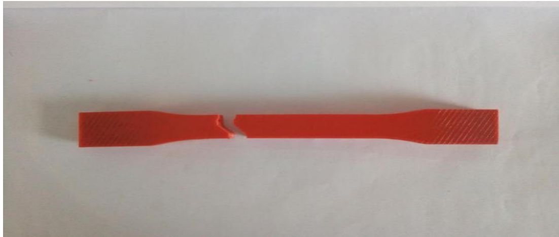
Figure 2. Tensile specimen of PLA after the test
