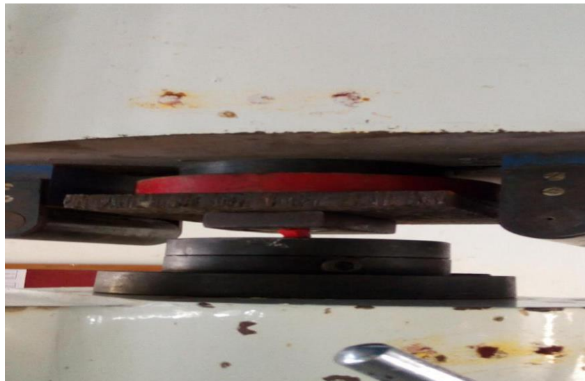
Figure 4. Compressive Strength Testing of PLA using UTM
