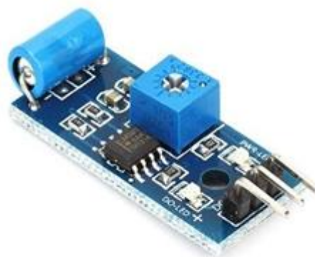
Figure 3.10: Arduino interface circuit for vibration sensor
