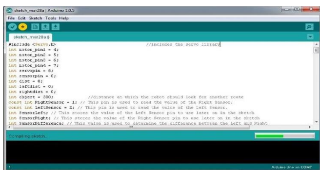
Fig 4.5 uploading the program Sketch to Arduino board
