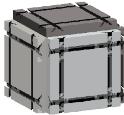
Figure 4. Contact pads are arranged symmetrically around four edges to perform rotational symmetry
