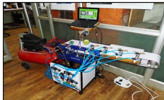
Figure 2. Machine vision based fruit sorter system
