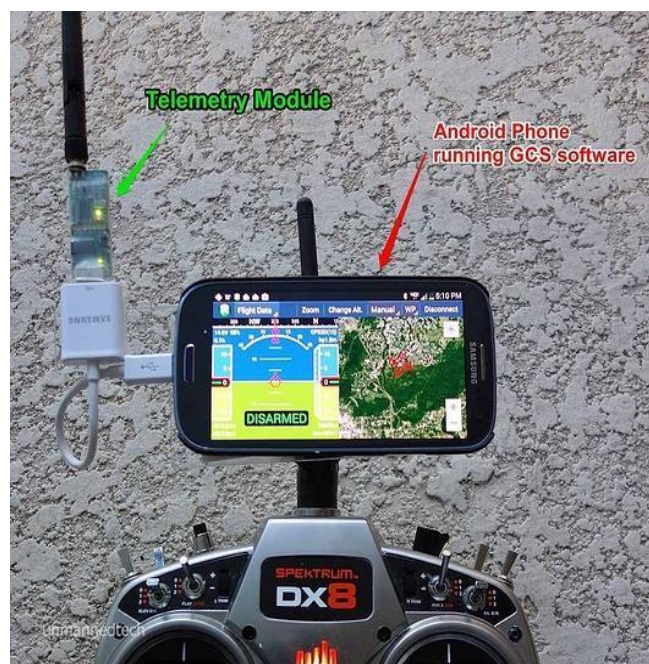
Fig. 5 Drone gcs telemetry. Base station connected with Mobile.
