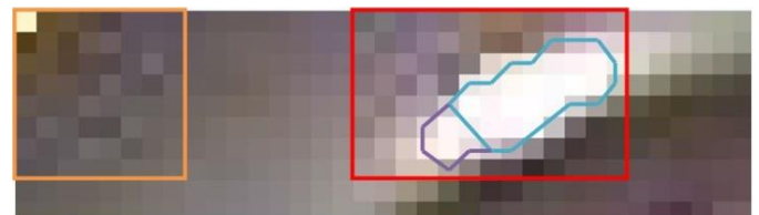
Figure 5 – JPEG file type generic image detail after edited only 3 (three) pixels and saved 20 (twenty) times. It is clear that the areas around the edited pixels have changed because of file compression calculation. Therefore, the original image data has changed, which can result negatively in the application of PADI.
