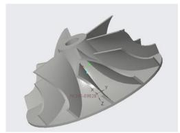
Fig 5: CAD Model of GARRETT GT-28 compressor
