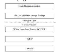
**Figure 4.** DICOM network communication protocols architecture.
