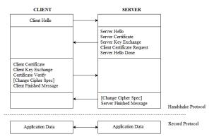
Figure 5. SSL Handshake between Client and Server
