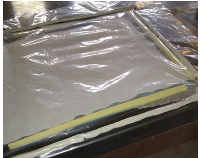
Fig 3. Vacuum bagging process
