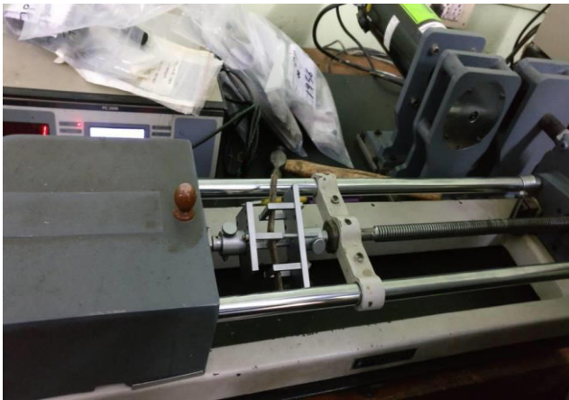
Fig 5. Tensile testing of the specimen
