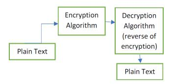
The above diagram describes the process of symmetric cryptosystem. This algorithm uses single key to convert information. Initially key will be shared among users.
